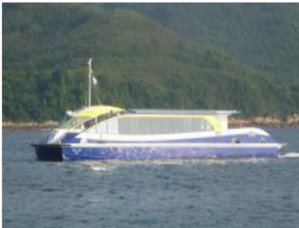
Figure 6.1: SolarSailor’s “Solar Golf” hybrid powered ferry (8% of energy from On-Board PV)
