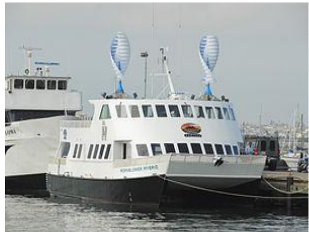
Figure 6.2: Hornblower Hybrid wind, solar and diesel ferry
