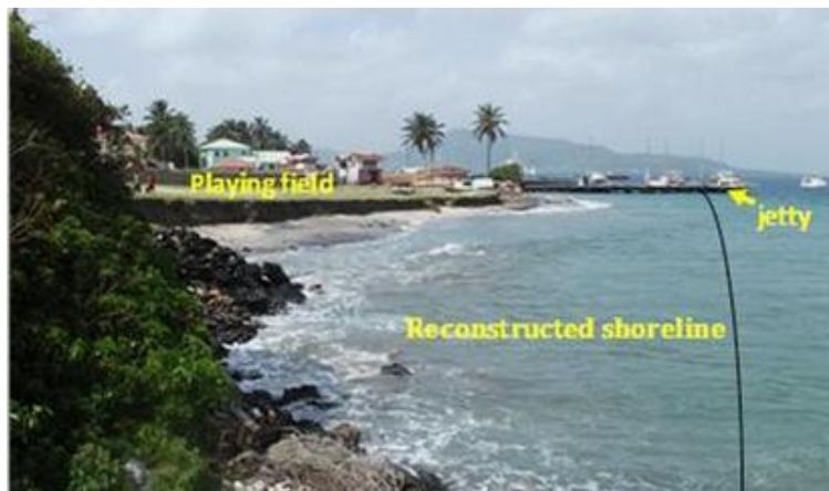
Figure 9.6: Erosion at Sanchez, showing the reconstructed 1960s’ shoreline (in black)
